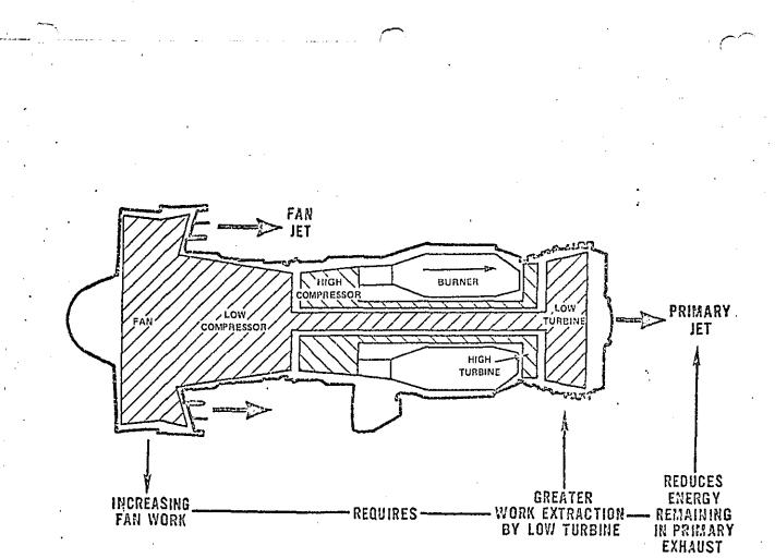
FIGURE 4. REFAN RETROFIT CONCEPT FOR JTED ENGINES.
